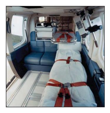
Cougar Helicopters currently operates the Bell 222U as its EMS platform primarily for the twin turbine power, extended operating range and high single-engine stay-up performance. The medical cabin was designed and installed by VIH Aviation Group and includes a proprietary double stretcher capability. The Bell 222U is particularly suited for scene responses and unprepared landing site operations.
